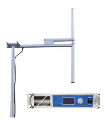
The transmitter implements digital FM modulator module as its core, combining with RF power amplifier. In the transmitter, DSP&DDS are used to execute all-digital processing, such as digital filtering, pre-emphasis, the generation of pilot frequency, stereo coding and FM modulating. A AGC circuit is used to keep the set power stable.
